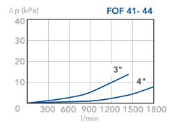
CLEAN FILTER ELEMENT PRESSURE DROP WITH F+, CC AND ME MEDIA (depending both on the internal diameter of the element and on the filter media)
